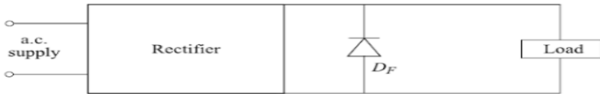
Fig.2.6: Position of commutating diode D_F
