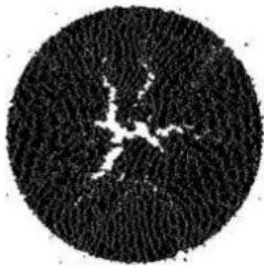
Cluster of microcracks in a melanin granule irradiated by a short laser pulse.
